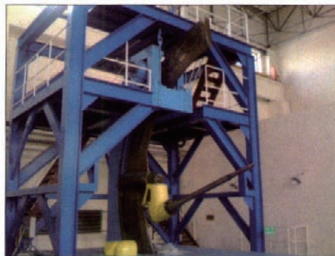
图8 FL-9风洞模型架车 Fig.8 Model support carriage in FL-9 wind tunnel
